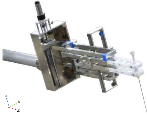
Fig.4 Produced end effector
