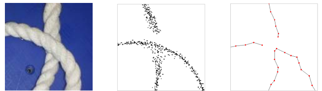
(a) Actual string shape (b) Center line point cloud (c) Point chain model
