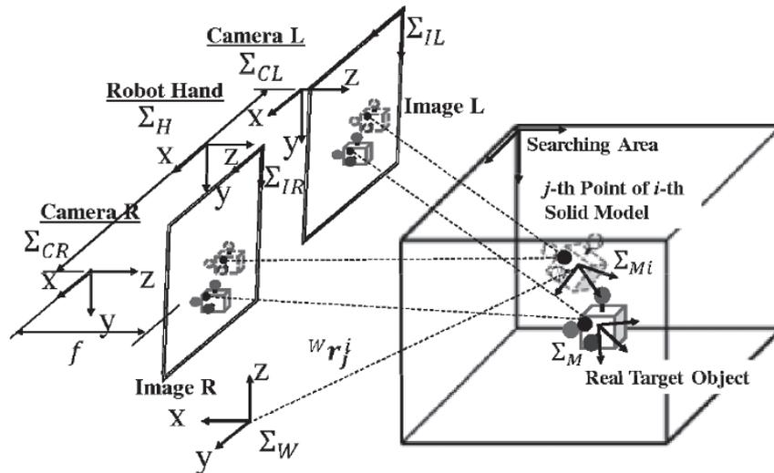
Fig. 1. Coordinate system of dual eyes – whose two cameras are set at the hand (represented by  $\Sigma_H$ ) of robot – are defined as  $\Sigma_{CL}$  and  $\Sigma_{CR}$ . The coordinates of camera images are  $\Sigma_{IL}$  and  $\Sigma_{IR}$ , in which real target object defined by  $\Sigma_M$  and  $i$ -th solid model defined by  $\Sigma_{Mi}$  are projected from the 3D space depicted at right side).
