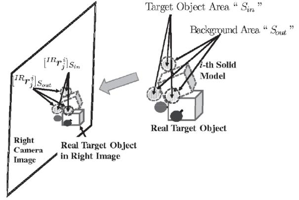
Fig. 3.  $i$ -th object model is projected to right image plane whose target object area denoted by “ $S_{in}$ ” and background area denoted by “ $S_{out}$ .” Projected points  ${}^{IR}r_j^i$  on “ $S_{in}$ ” are represented as  $[{}^{IR}r_j^i]_{S_{in}}$  and on  $S_{out}$  as  $[{}^{IR}r_j^i]_{S_{out}}$ .
