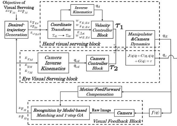
Fig. 4. Block diagram of the hand visual servoing system.
